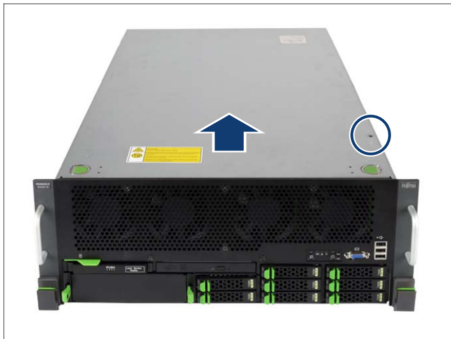
Figure 44: Opening the server
